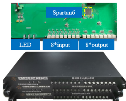
Figure 7: The interlocking fan-out electronics hardware.
