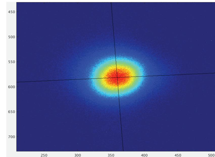
SR from 1st arc dipole ("round beam")  $\rightarrow$
