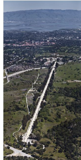
3 km linear accelerator at SLAC, \Delta E = 17 MeV/m 3 / 1
