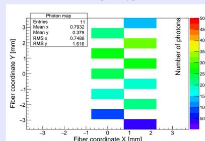
2D vertical beam measurement by optical fiber + MPPC readout
