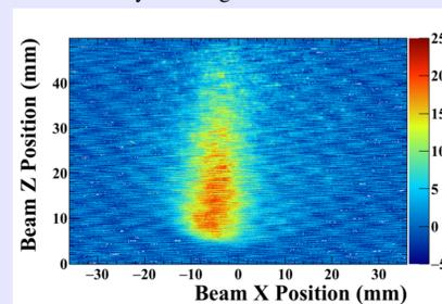
2D horizontal beam measurement by Image Intensifier + CID camera
