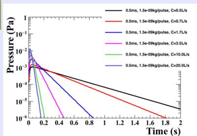
Expected pressure vs. time for different gas injection valve conductances
