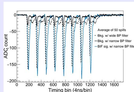
Observed beam-induced background on an optical fiber before and after background mitigation (with optical filtering of 400±200 nm and 400±40 nm respectively) and observed BIF signal after mitigation
