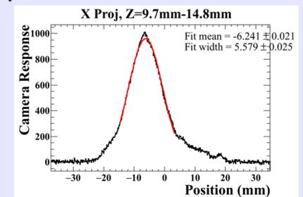
1D horizontal beam measurement by Image Intensifier + CID camera
