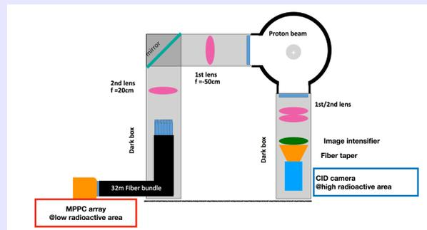
Schematic diagram of the BIF monitor optical systems.
