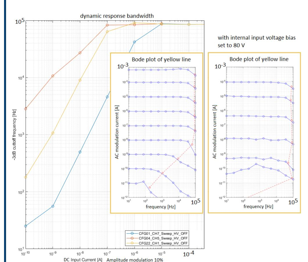
• With lower currents, the sensitivity to <u>noise</u> increases. A plot of a 10% current modulation (below) is showing strong noise at a DC current of 1 nA.
