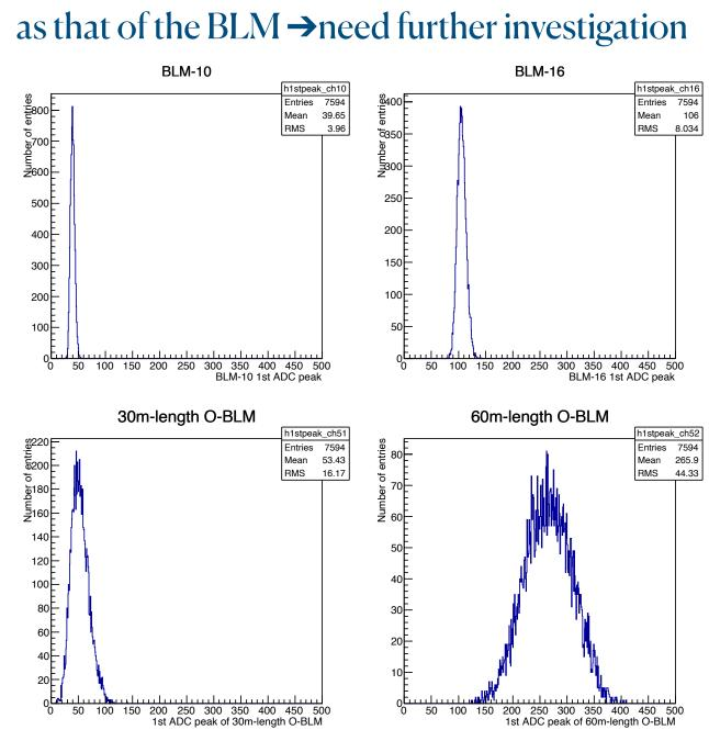
BLM-10 (16) are at the most upstream (downstream) of the 60 m-length O-BLM respectively. BLM-01 (50) are 30 m upstream away and 190 m downstream from the O-BLM respectively. Data taken in ~ 5hours.
