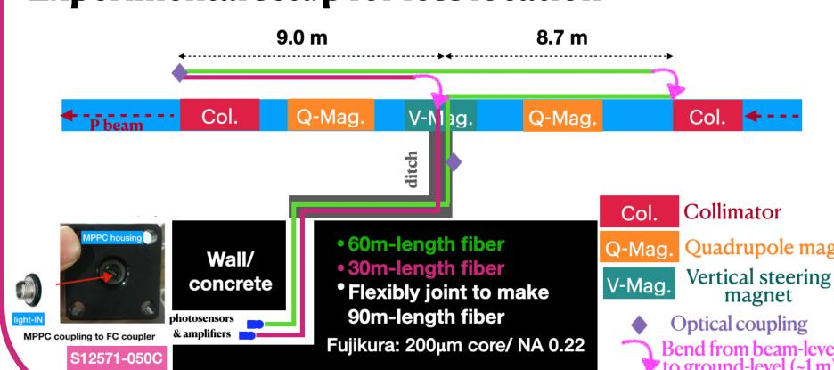
• MPPC is not rad-hard; fiber is guided to sub-tunnel
