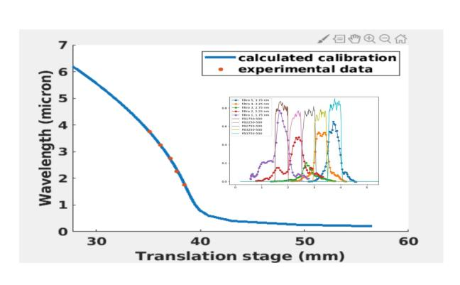
The spectrometer is wavelength calibrated by means of IR band pass filters and analytic description.
