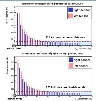
Response distributions for various positions of RMS-R3 modules with respect to the beam pipe along X (top) and Y (bottom) axis
