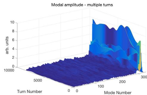
Figure 5: Measurement from the Dimtel feedback system, showing unstable modes over ~9,000 turns.
