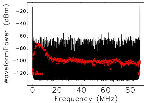
Figure 4: Example spectrum analyzer measurement for 324 bunches. The full measurement is shown by the black lines and is dominated by revolution harmonics; peaks at the lower vertical betatron sidebands are shown as red diamonds.
