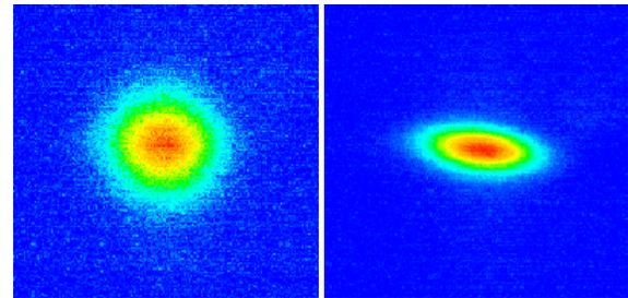
Figure 3: Pinhole camera images. Left: one train with no gaps; the beam is blown up vertically due to ion instability. Right: 4 trains with gaps; the instability is suppressed.
