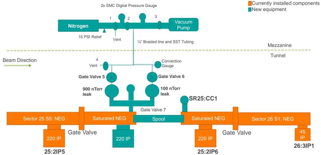
Figure 1: Layout of gas injection system.
