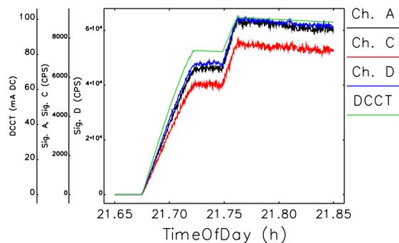
Figure 6: Gas bremsstrahlung detector measurement. Each channel corresponds to a different photon energy threshold.
