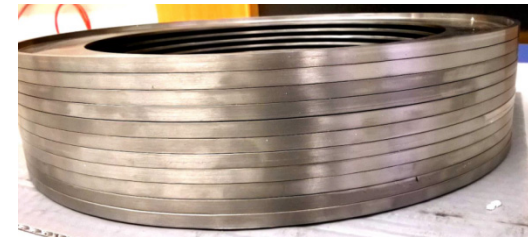
Inner and outer segments welded
