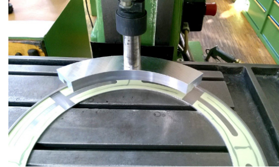
Fixation of GFK spacers
