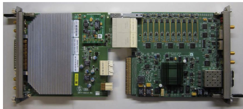
Struck transition module, Digitizer w/Xilinx KU in MTCA Also, custom RF front end
