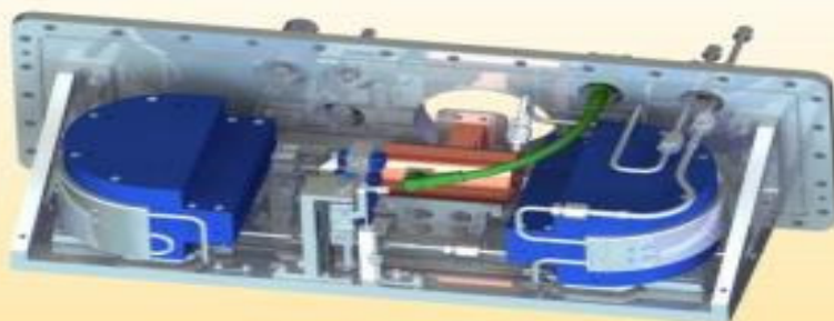
3D image of the interior of the accelerator head / vacuum chamber
