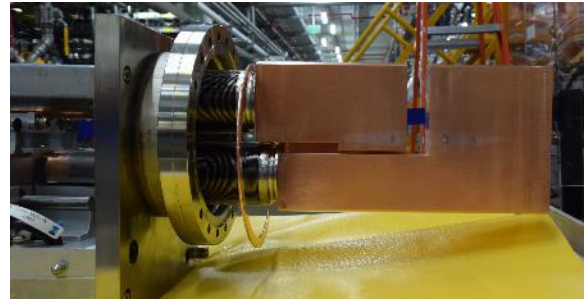
Figure 1: FRIB LPCS with visible radiation damage.
