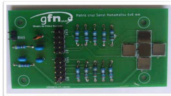
Cross Array 2x2 MicroFJ-60035 ( SensL )
