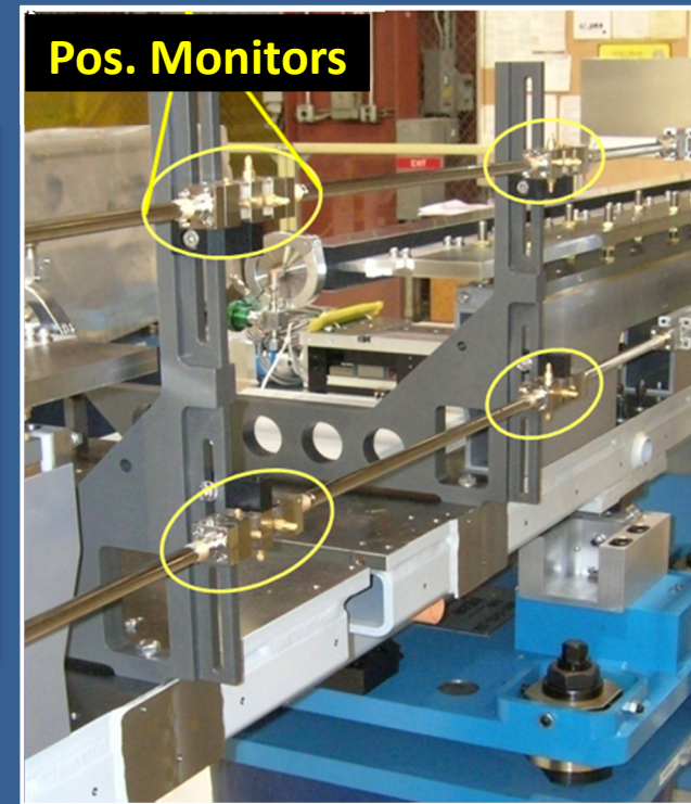
Position diff's of 33 undulators after 47 days of operation
