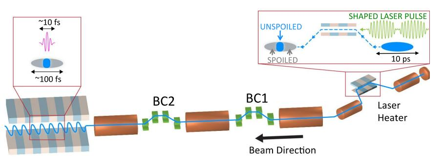
Coherent2 Heater Pulse Ti:Sa  $\lambda$  = 760 nm Bandwidth ~4 nm FWHM Heater stretched to ~16 x Fourier limit  $\Delta T$  ~ 8 ps  $\Delta T_{coh}$  ~ 360 fs Use DAZZLER to shape Heater
