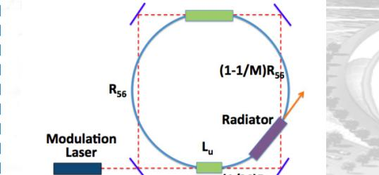
A possible technique for generating high average power coherent EUV radiation
