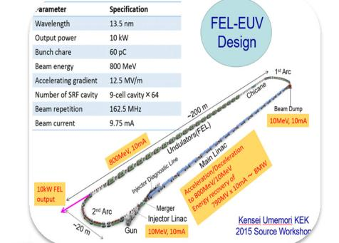
Superconducting energy-recovery linac (ERL)
