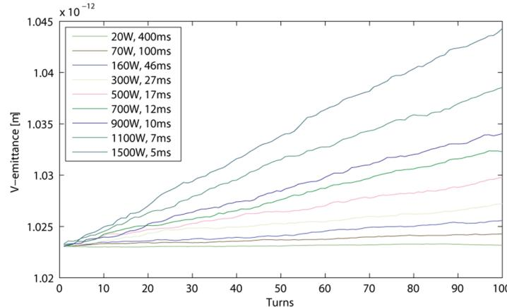
Vertical emittance growth for different average output power and corresponding growth time, for high output peak power, the longitudinal phase space is significantly changed after the radiator
