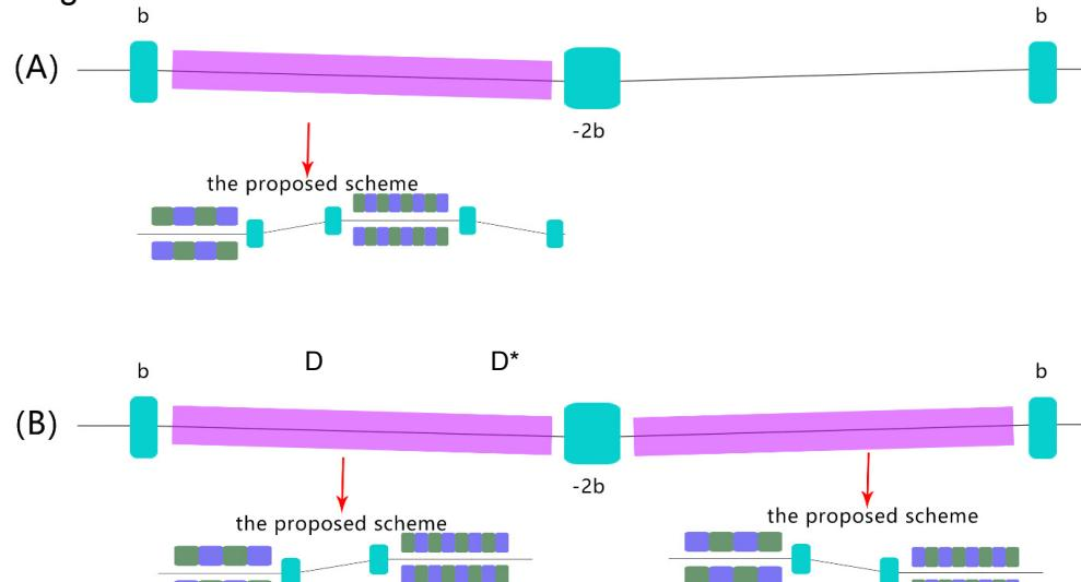
Two possible lattices in the long drift section of SR
