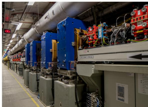
Figure 1: First bunch compression chicane.
