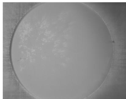
Figure 5: Image of the dense array above in the AZO coating. We suspect in this case the insulating diamond substrate charged and damaged the coating during discharge.
