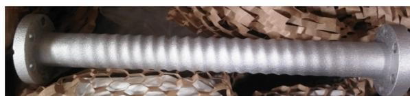
Figure 7: A 34 GHz  $TE_{11}$ - $TM_{01}$ - $TM_{11}$  RF undulator.
