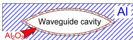
Figure 2: Cross-section of FEL waveguide.
