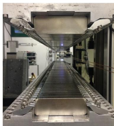
Figure 5: New Modulator Magnetic Array.
