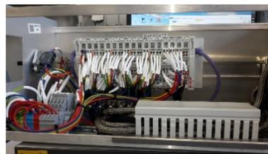
Figure 6: Assembly of a PLC module at NCBJ.
