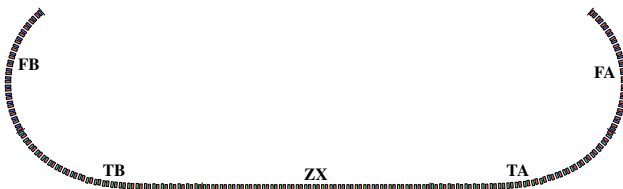
Figure 4: The FFA return arc, showing individual magnets. Red magnets are the focusing quadrupoles, other magnets are defocusing, the color indicating which type of defocusing magnet is used. FA and FB contain the arc cells, ZX contains the straight cells, and TA and TB contain the cells making up the adiabatic transition.
