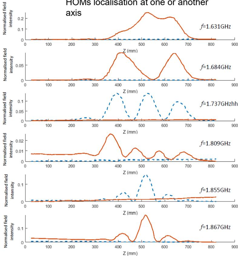
The RF coupler is located on one axis (active) while the field measurements are conducted on both axes
