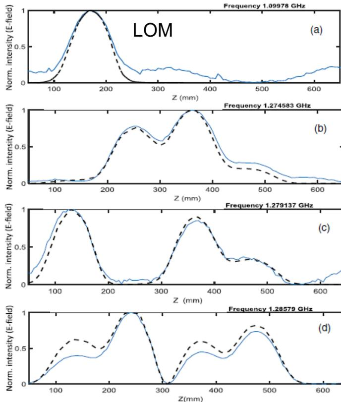
First comparison of the pass band modes measured (solid line) with the numerical predictions dashed line. The measurements were carried out at a single axis.
