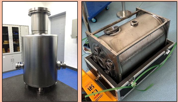
KEK-B type 1-cell 500MHz SRF cavity
