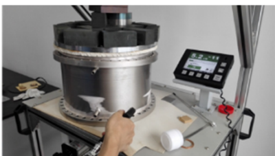
Vacuum leak detection
