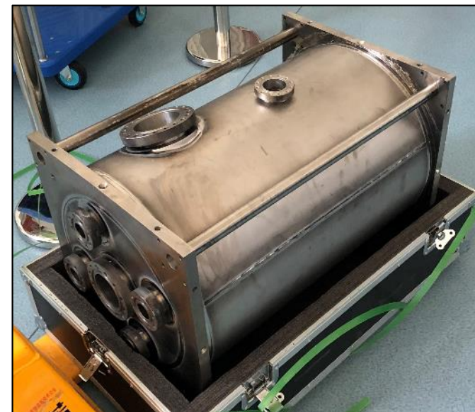
He vessel welded
