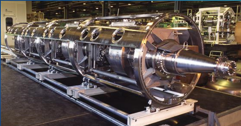
4-cavity CM without MLI and outer vessel
