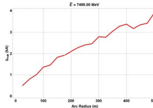
For this example **considering only the peak current** we should pick arc radius of 150 m to ensure ISR limit lies above 1.5 kA
