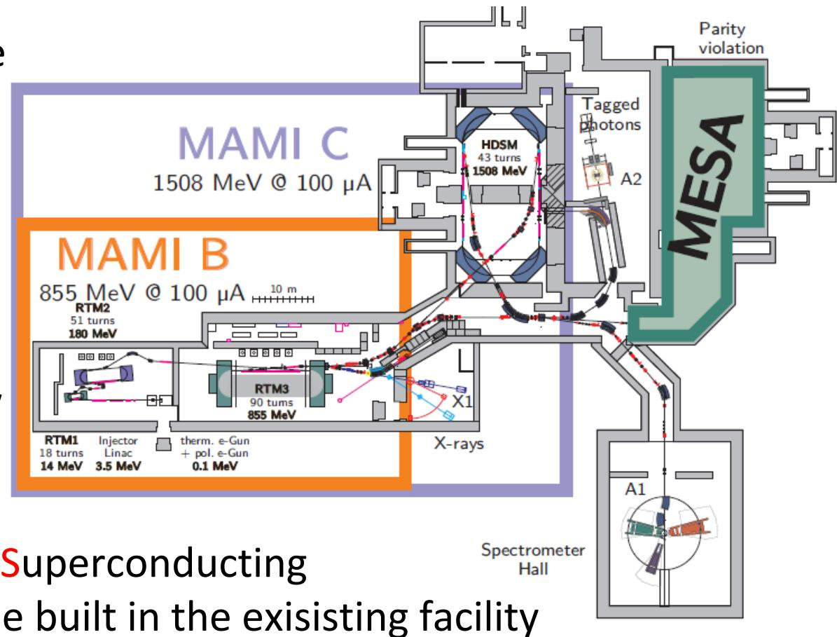
Mainz Energy Recovery Superconducting Accelerator (MESA) to be built in the existing facility
