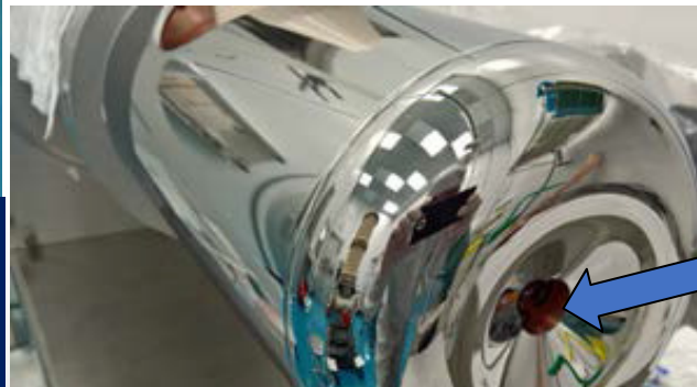
Molybdenum cathode plug
