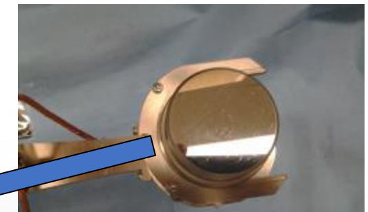
Molybdenum cathode plug
