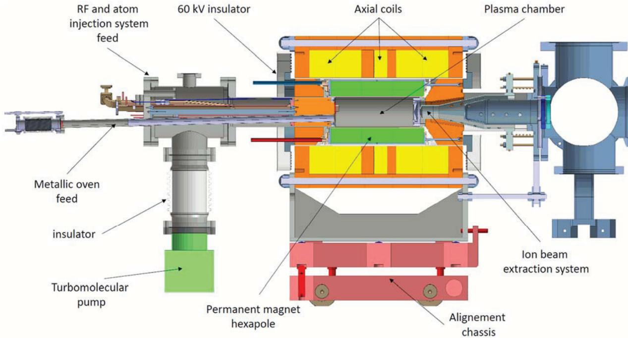
Figure 1: Sectional view of the PHOENIX V3 ion source mechanics.
