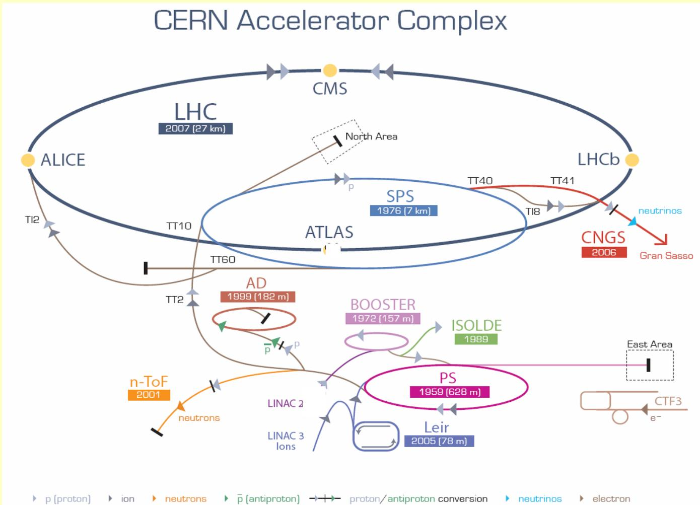
LHC Large Hadron Collider SPS Super Proton Synchrotron PS Proton Synchrotron
