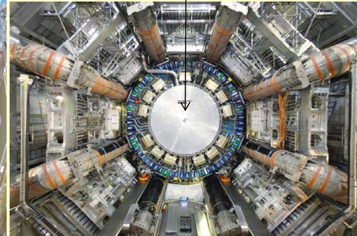
VA vacuum beam pipe installed before closure of the endcap
