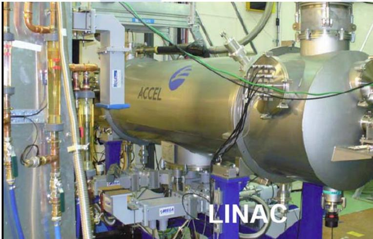
Linac and booster both consist of two TESLA 9 cell cavities in a Rossendorf/Stanford module
