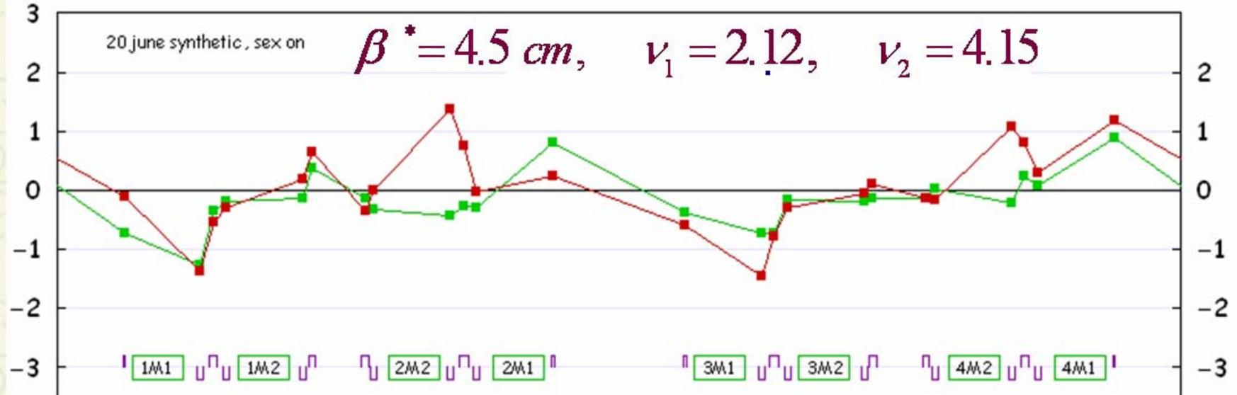
☛ Orbit response matrices on dipole and quadrupole corrections + Singular Values Decomposition
