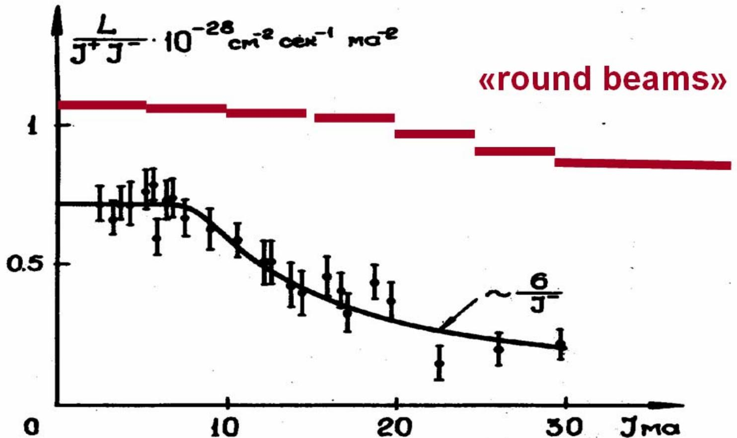
Specific luminosity versus electron beam current
