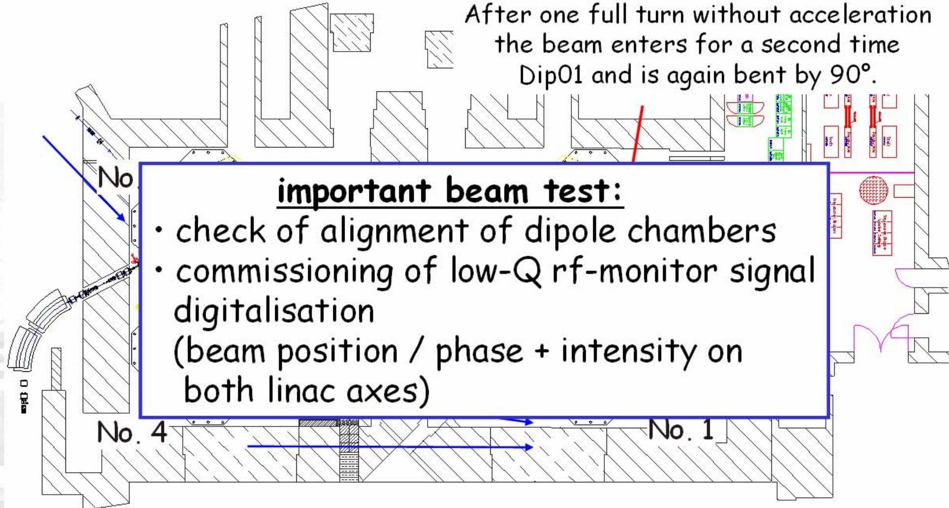
Field in Dip03+04 reduced by  $\sim 9\text{MeV}/855\text{MeV} = 1.05\%$
