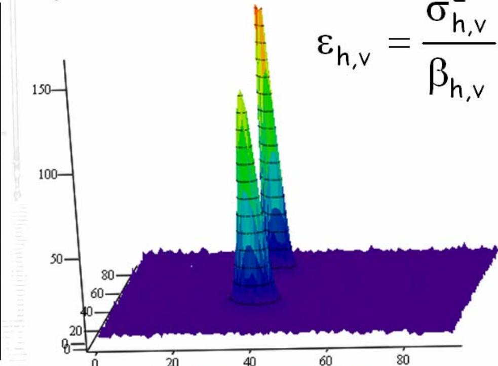
$$\sigma_v = 2.05 \text{ pix} = 0.279 \text{ mm}, \\ \beta_v \sim 40.3 \text{ m}$$
