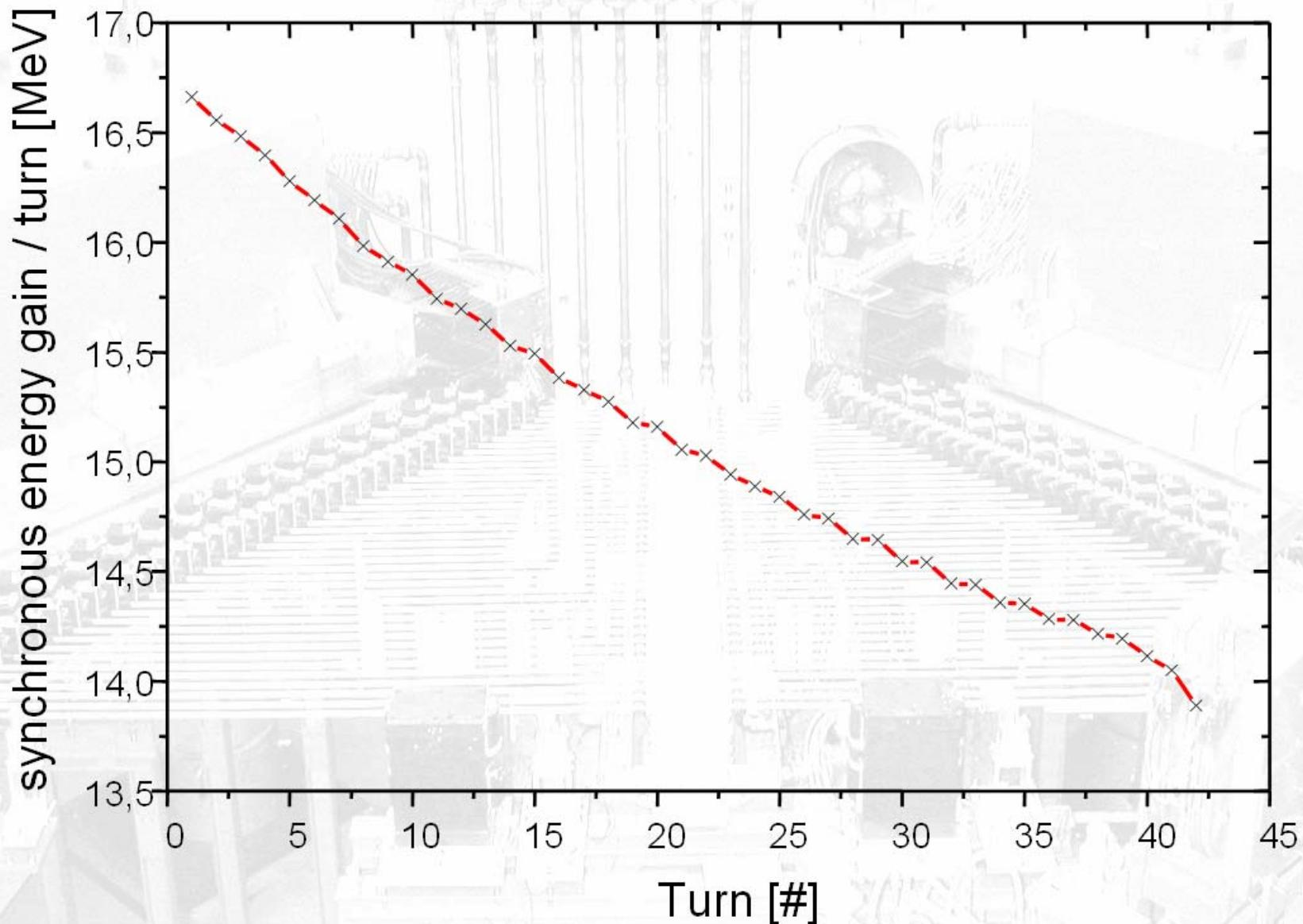
With increasing energy the beam intrudes deeper and deeper into the 90° dipoles and experiences, compared to a homogenous dipole, turn by turn a relatively decreasing field-integral, which requires less energy gain per turn to fulfil the dynamic coherence condition.
