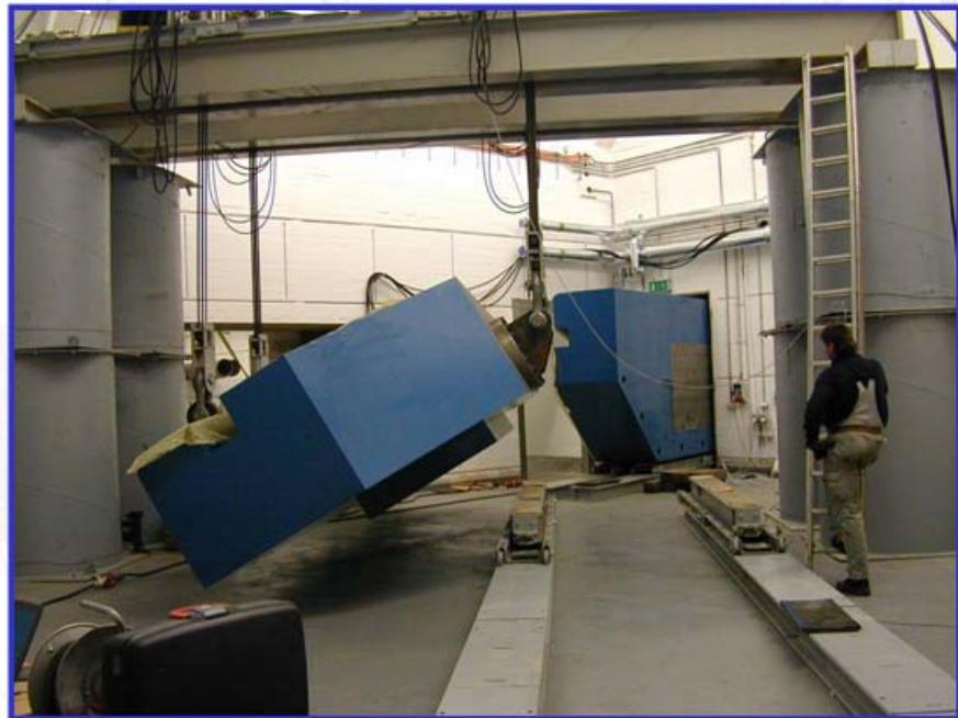
measurement of the magnetic field of all 4 magnets to get the data for the construction of surface correction coils
