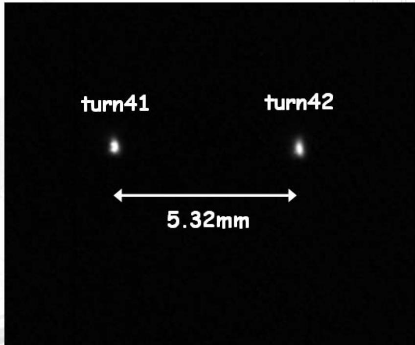
$$\sigma_h = 2.215 \text{ pix} = 0.301 \text{ mm}, \\ \beta_h \sim 7.4 \text{ m}$$
