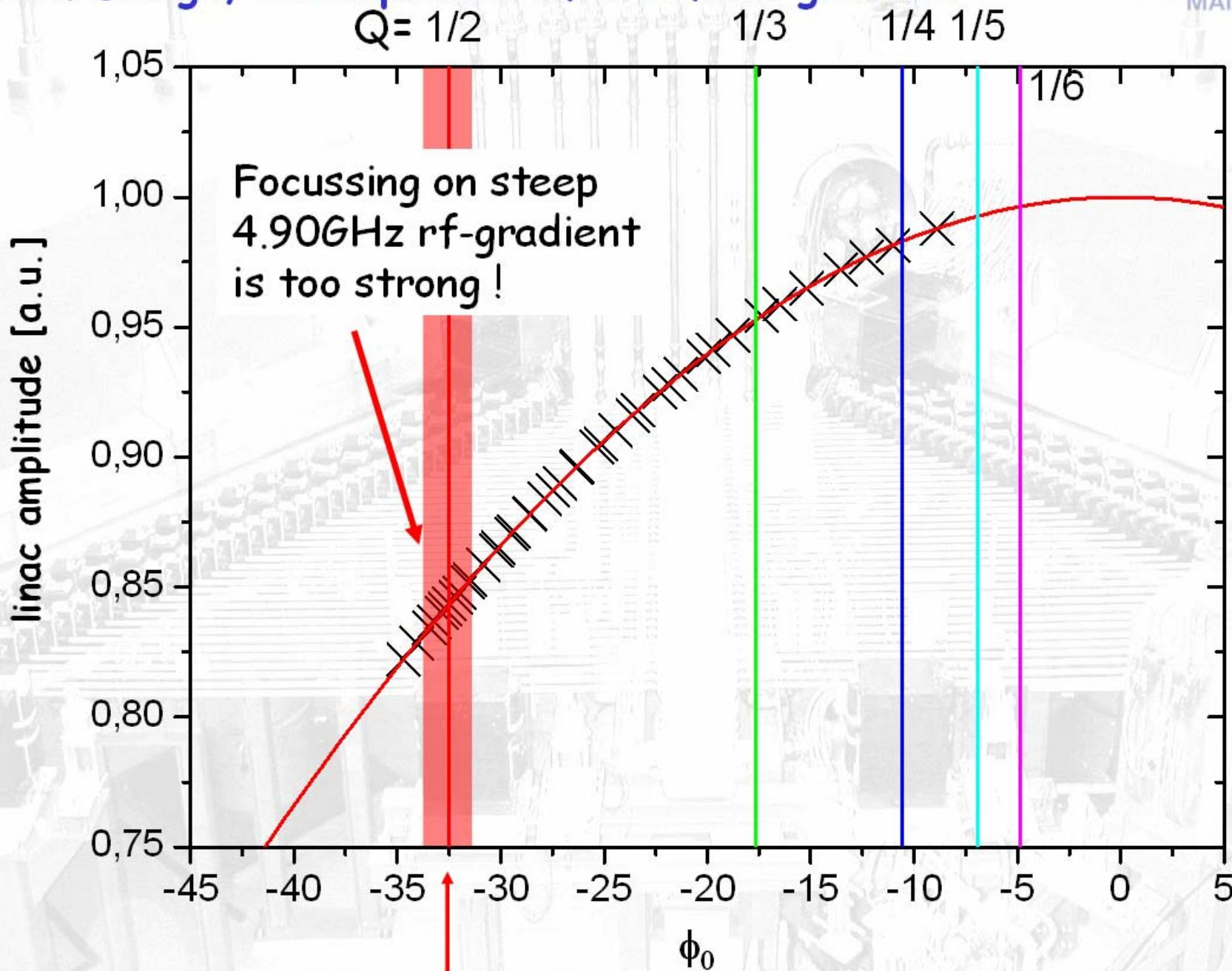
stop band when certain phasing error between linac 1 and linac 2
