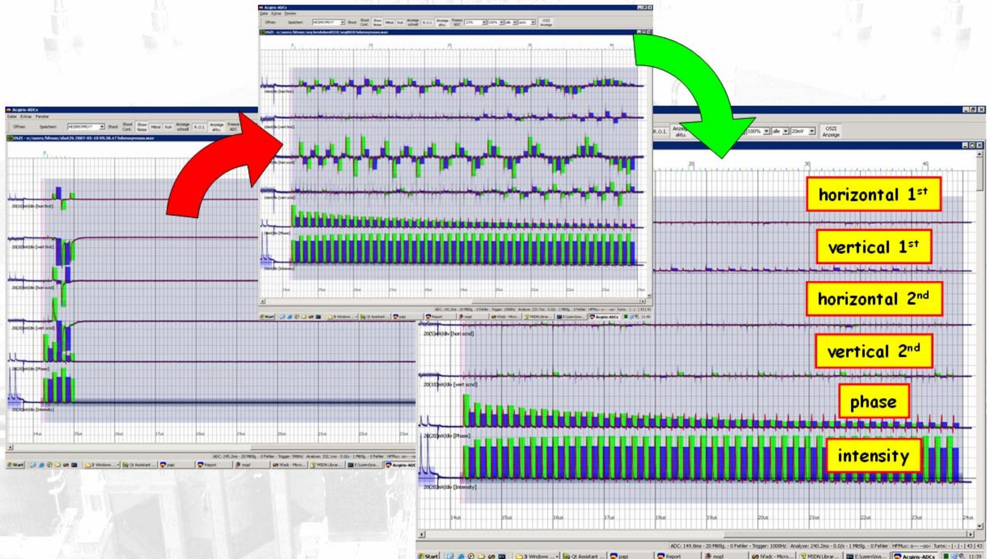
signals of low-Q rf-monitors of both HDSM-linacs
