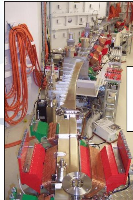
Assembly of the complete sector over the open magnets.
