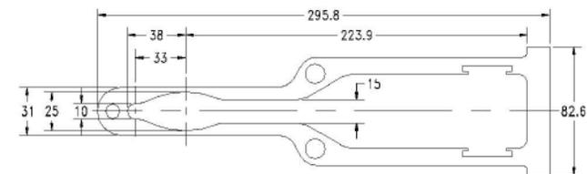
Dipole chamber extruded cross sections
