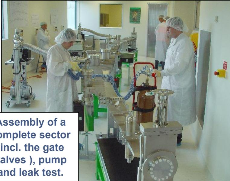
Assembly of a complete sector (incl. the gate valves), pump and leak test.
