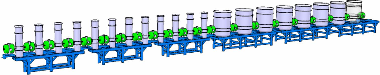
**SPIRAL-2 philosophy** : Smoothest beam dynamics (regular FDO lattice, low number of  $\beta$ -sections), Modular solution and simple cryostats, Separated vacuum (safety with FP), Warm focusing (easier for alignment), Possibility to insert diagnostics at each period, ease of tuning
