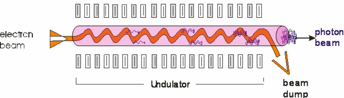
Narrow-band amplifier with resonance wavelength:
