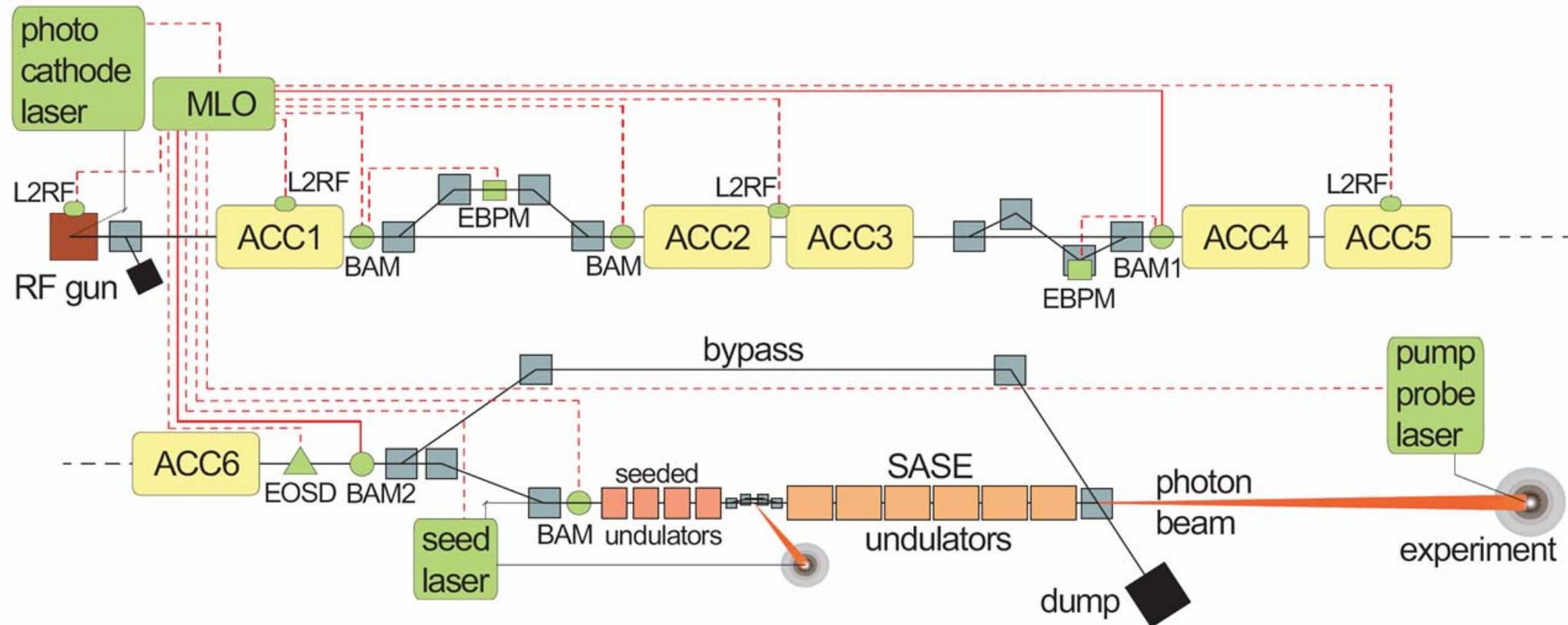
A sub-10 fs stable optical synchronization system is currently being developed at FLASH.
