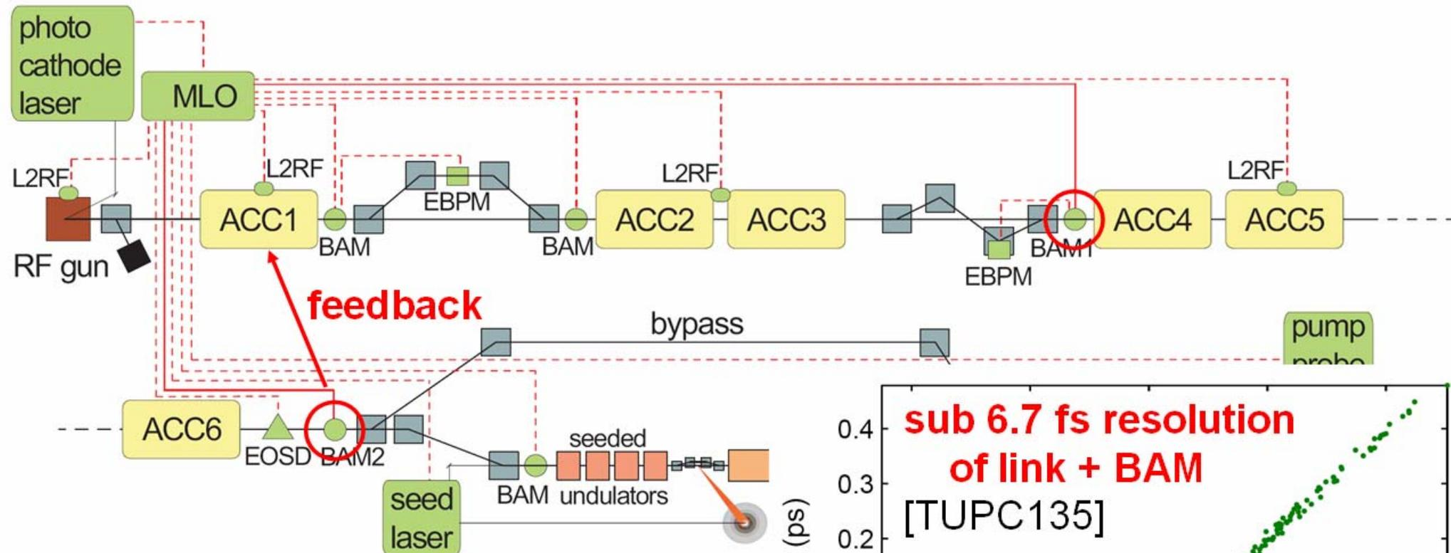
Arrival time measurement with two BAMs in a straight section.
