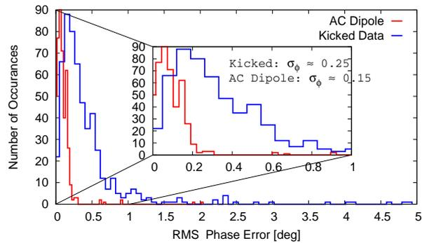
Figure 7: Histogram of the rms phase noise from all the BPMs from several data sets both from kicked data and ac dipole excited data.
