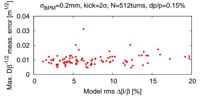
Figure 3: Maximum error in  $ND$  measurement vs. rms  $\beta$ -beating (simulation) for a 100 of LHC machines with errors.
