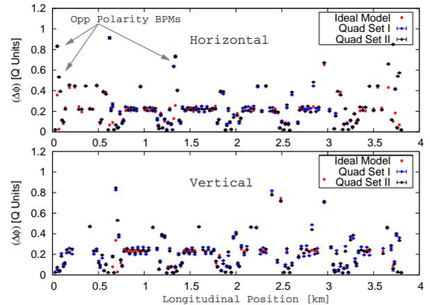
Figure 4: Measured phase advance between RHIC BPMs after trimming 1<sup>st</sup> set of three quadrupoles (blue) and the 2<sup>nd</sup> set (black) compared to the ideal model (red). Vertical error bars are statistical deviation between three consecutive data sets with the same condition
