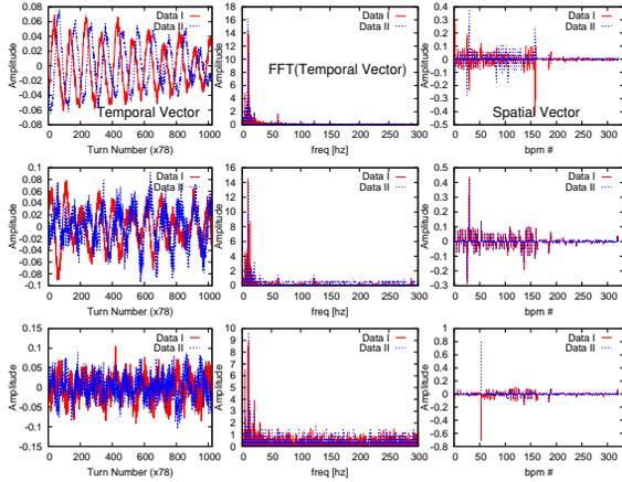
Figure 5: Sample correction of two difference orbits from the acquired data. Correctors near IR10 are appear to correct the RMS orbit by a factor of 3 or better in the Blue ring for both samples.
