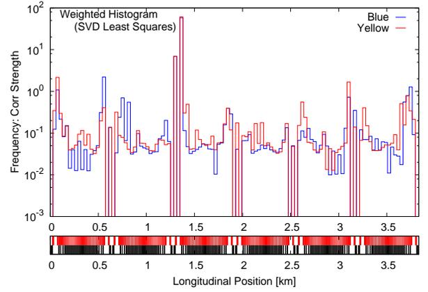
Figure 6: Top: Histogram of orbit correctors weighted by their strength to correct the difference orbits obtained from the 1 kHz acquisitions accumulated over several difference orbits ( $d_j$ ) and data sets ( $D$ ).
