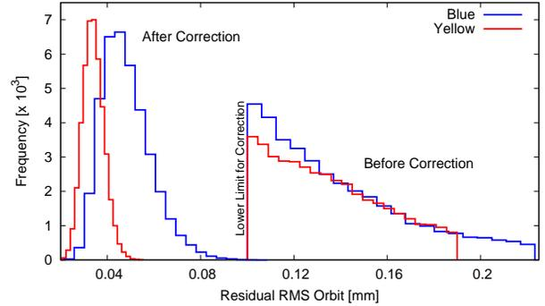
Figure 7: Histogram of the residual rms orbit before and after correction in both the rings.
