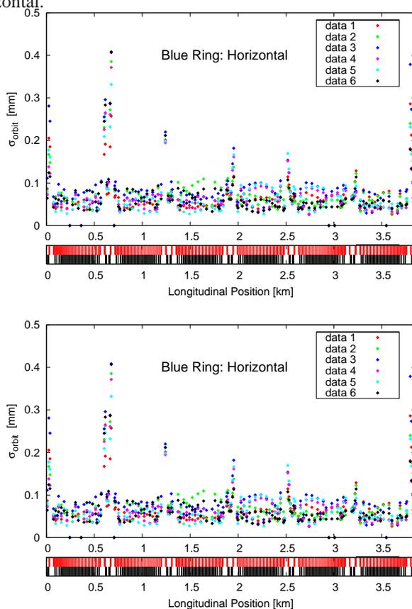
Figure 1: Top:  $1\sigma$  deviation of 1024 orbits each acquired from single turn sampled at 1 kHz is plotted as a function of longitudinal position for the Blue ring.
