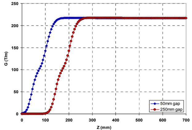
Figure 2: Longitudinal variation of field gradient between magnets.
