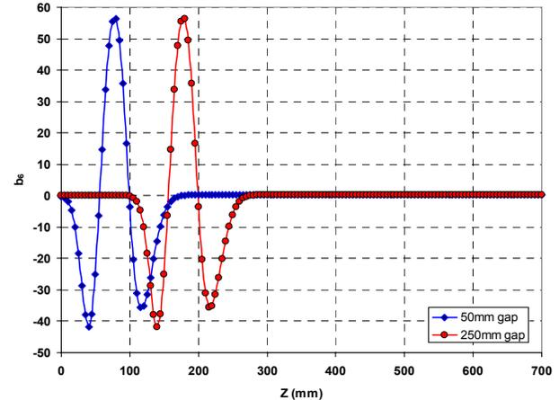
Figure 3: Longitudinal variation of  $b_6$  between magnets.
