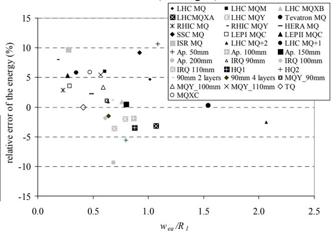
Figure 3: Agreement between numerical estimate of magnetic energy and analytical estimate for a 30° sector coil based on (10).
