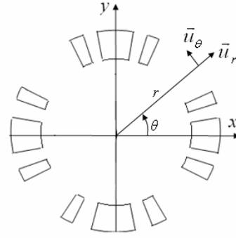
Figure 1: Cross-section of a Quadrupole magnet made of 2 pure sectors.
