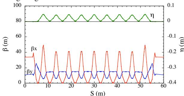
Figure 8: Betatron and dispersion functions in a cell for high emittance optics.
