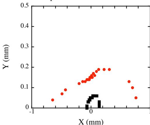
Figure 7: Dynamic aperture before harmonic correction ■ and after harmonic correction ● for low emittance optics.
