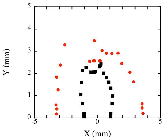
Figure 9: Dynamic aperture before harmonic correction ■ and after harmonic correction ● for high emittance optics.
