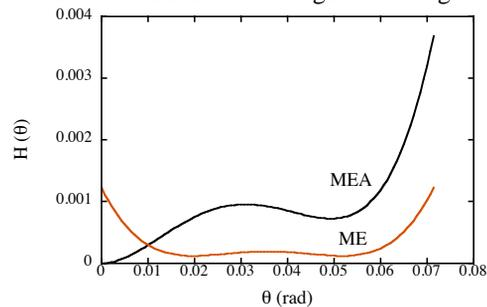
Figure 1: H-functions of SPring-8 bending magnet for minimum emittance (ME) and minimum emittance achromat (MEA) condition.
