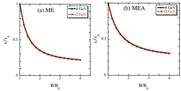
Figure 3: Normalized emittance of ME and MEA for the case of second order polynomial.
