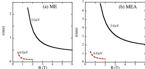
Figure 2: Emittance of ME and MEA for the case of second order polynomial.
