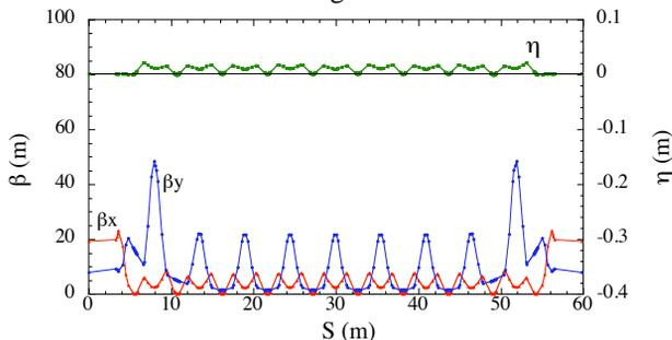
Figure 6: Betatron and dispersion functions in a cell for low emittance optics.
