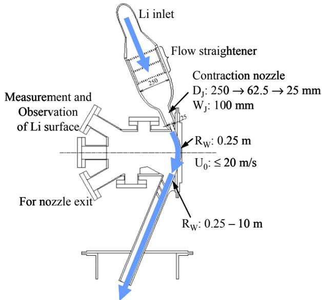
Figure 4: Schematic view of the liquid lithium target. After purification, the lithium is injected on the backplate thanks to a nozzle, which contracts the flow thickness from 250 down to 25 mm. The width of the lithium flow, perpendicular to the Figure, is 260 mm.
