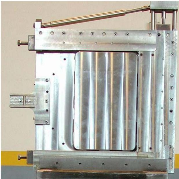
Figure 5: photograph of the bayonet backplate, designed by ENEA.
