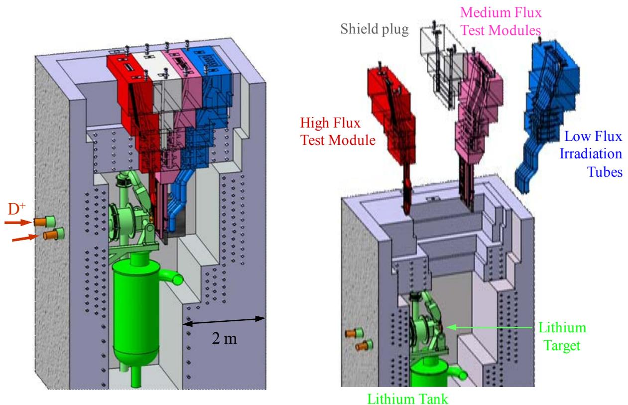
Figure 6: Cut of the Test Cell with the Modules in position (left part of the figure) or out of it (at the right).
