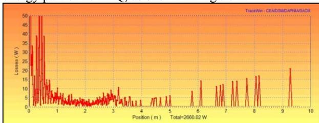
Figure 2: Beam losses (in Power) along the LEFT Case of an unmatched beam coming from the LEBT
