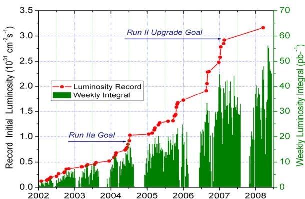
Figure 1: Tevatron peak and weekly integrated luminosity in 2002-2008.
