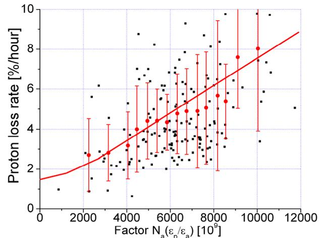
Figure 2: Proton-bunch intensity loss rates at the beginning of the Tevatron stores (FY08) vs factor  $F$ .
