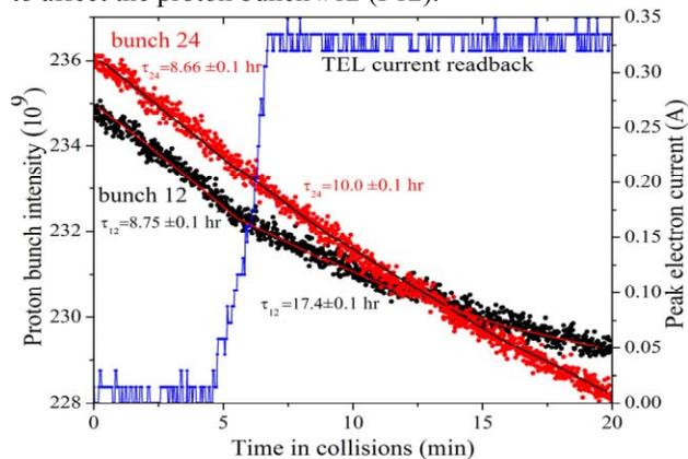
Figure 4: Effect of TEL2 on proton intensity decay.
