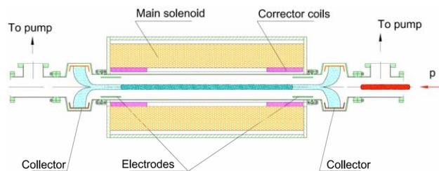
Figure 9: Electron column for space-charge compensation.
