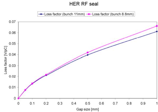
Figure 5: Loss factor of a sealed cavity.
