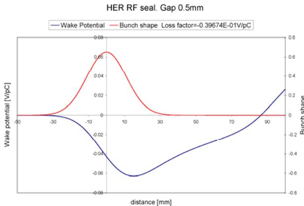
Figure 4: Wake potential of a 11 mm bunch.
