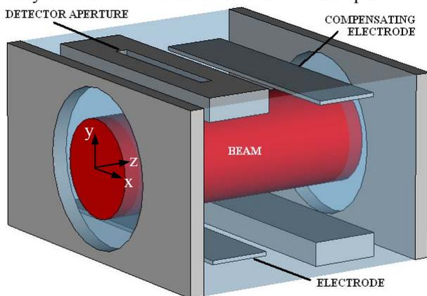
Figure 1: RGI profile monitor geometry
