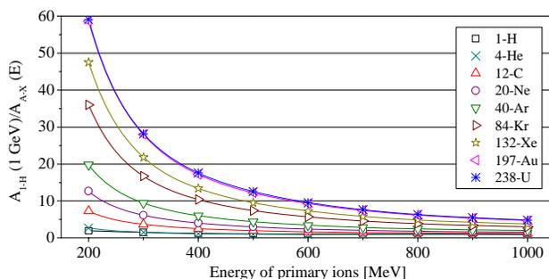
Figure 5: Scaling factor for the beam-loss tolerance as a function of projectile energy.  $A_{1-H}(1\text{GeV})$  is the normalized activity induced by one 1 W of 1 GeV proton beam,  $A_{A-X}(E)$  is the normalized activity induced by 1 W of ion beam of interest at given energy. The activities are calculated by FLUKA immediately after the end of irradiation in copper.
