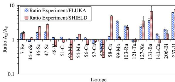
Figure 1: Ratio  $A_E/A_S$  for the isotopes with dominating contribution to the residual activity in stainless steel irradiated by 950 MeV/u 238-U ions.  $A_E$  is the experimentally measured activity and  $A_S$  is the activity calculated by FLUKA and SHIELD.
