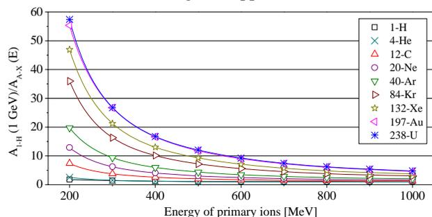
Figure 4: Scaling factor for the beam-loss tolerance as a function of projectile energy.  $A_{1-H}(1\text{GeV})$  is the normalized activity induced by one 1 W of 1 GeV proton beam,  $A_{A-X}(E)$  is the normalized activity induced by 1 W of ion beam of interest at given energy. The activities are calculated by FLUKA immediately after the end of irradiation in stainless steel.
