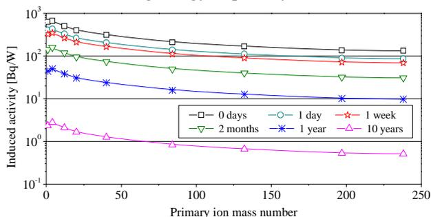
Figure 2: Activity per watt induced in stainless steel by different primary ions at 1 GeV/u calculated by FLUKA .
