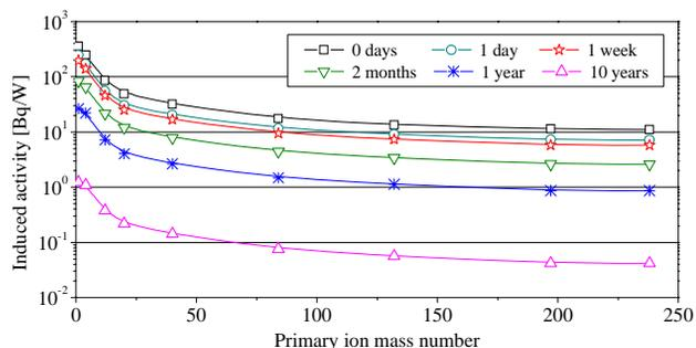
Figure 3: Activity per watt induced in stainless steel by different primary ions at 200 MeV/u calculated by FLUKA.
