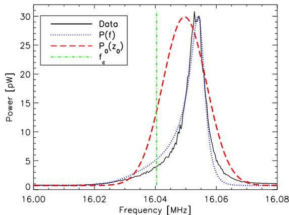
Figure 4: Vertical upper Schottky band of the 75<sup>th</sup> harmonic. The beam parameters are the same as in Fig. 3.
