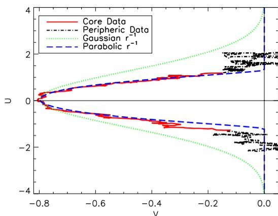
Figure 1: Stability diagram of the upper sideband of the 98<sup>th</sup> harmonic in the vertical plane. For beam parameters see Tab. 1. Core data is called what defines almost the entire shape of the stability diagram but only the center of the BTF's amplitude in Fig. 2.
