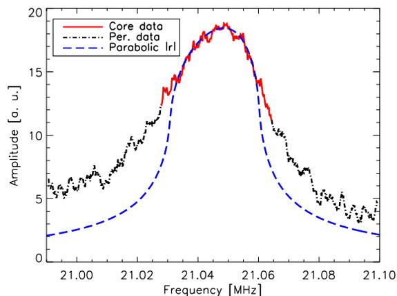
Figure 2: Amplitude of the BTF measured at the upper sideband of the 98<sup>th</sup> harmonic in the vertical plane. The parabolic BTF matches the data only in the range that is relevant for the stability diagram (Fig. 1). The peak has a slight asymmetry that we refer to the space charge. The best agreement for the parabolic distribution was found for  $\Delta U_{fit} = -0.06$ .
