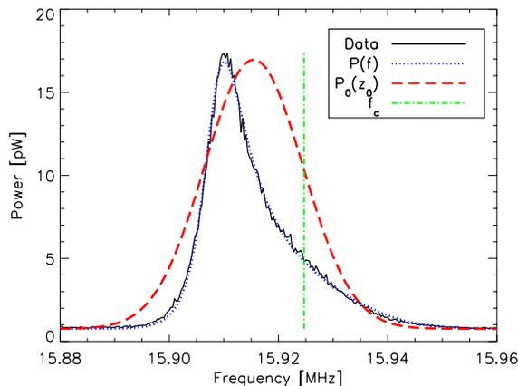
Figure 3: Vertical lower Schottky band of the 75<sup>th</sup> harmonic. For beam parameters see Tab. 1.  $P$  is the fit of Eq. (5) to the data.  $P_0$  was computed with the parameters from the fit and shows what the band would look like in the absence of space charge.  $z_0$  is equal to  $z$  [Eq.(4)] for  $\Delta Q = 0$ . The vertical straight line shows  $f_c$  obtained from the fit. It is shifted off the center of  $P_0$  by the incoherent space-charge effect.
