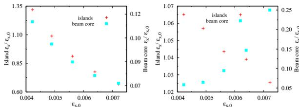
Figure 5: Relative islands emittance as a function of the initial emittance. Two types of tune curves are used: 1 – 1 (left) and 2 – 3 (right).
