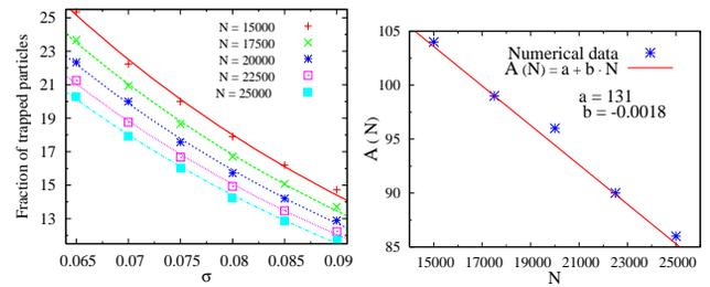
Figure 6: Fit results of the fraction of trapped particles as a function of the total number of turns  $N$  with an exponential function (left). The amplitude of such an exponential is fitted as a linear function of  $N$  (right).
