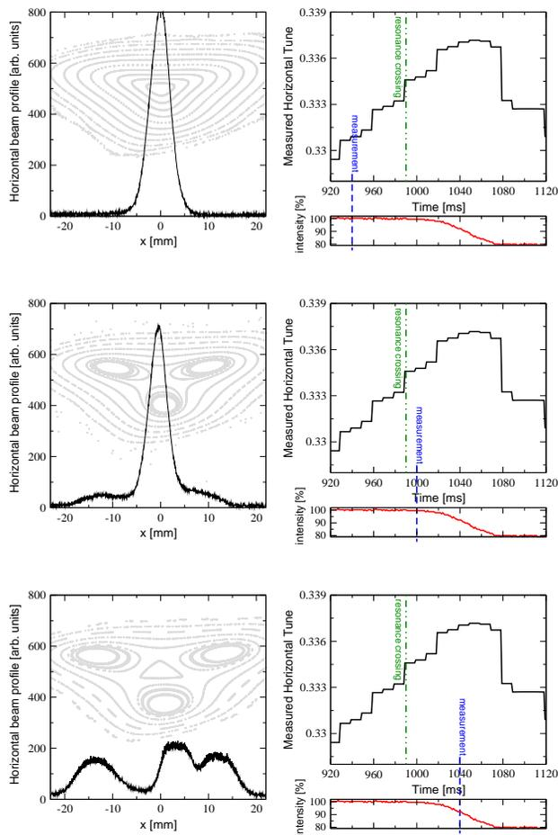
Figure 2: Evolution of the horizontal beam profile during the crossing of the one-third resonance. The profile is shown before the resonance is crossed (upper), right after the crossing (centre), and at the end of the crossing (lower). The corresponding phase space portrait obtained from the MADX PS model is superimposed to the measured profile.
