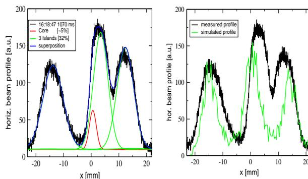
Figure 3: Measured horizontal beam profile at the end of the capture with superimposed multi-Gaussian fit (left), and comparison with multi-particle MADX simulations including chromaticity and tune modulation (right).
