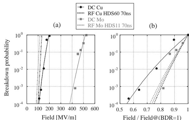
Figure 4: Breakdown probability of Cu and Mo in DC and in RF tests, (a) vs applied field, (b) vs normalized field.
