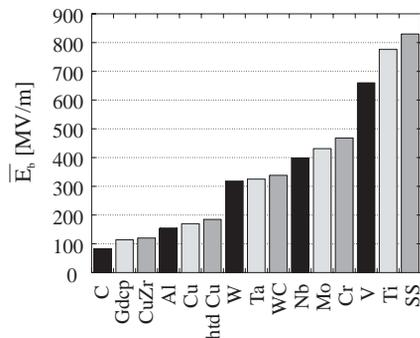
Figure 2: Saturated breakdown field  $\overline{E}_b$  of tested materials.
