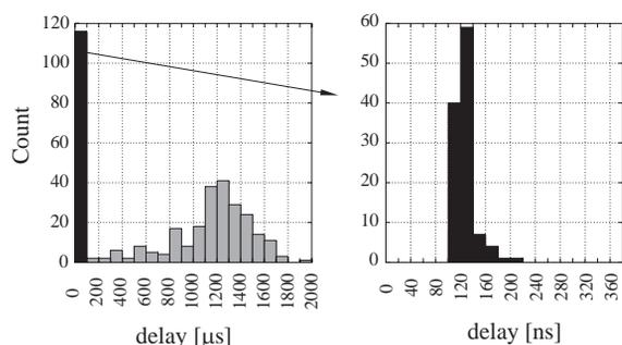
Figure 5: Histograms of delays with Mo electrodes.
