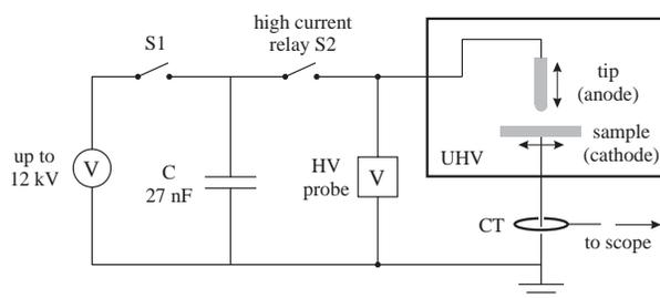
Figure 1: Schematic drawing of the experimental setup.
