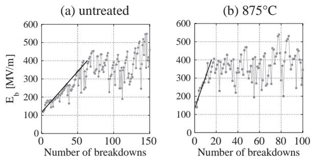
Figure 3: Improvements in conditioning speed of Mo after a heat treatment.
