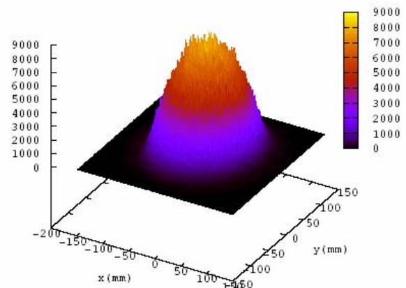
Figure 1: Beam profile (W/cm<sup>2</sup>) at the beam dump entrance.
