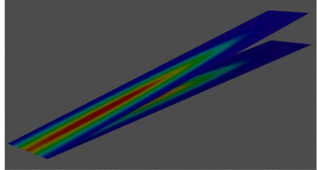
Figure 3: Power deposition in plates beam dump.
