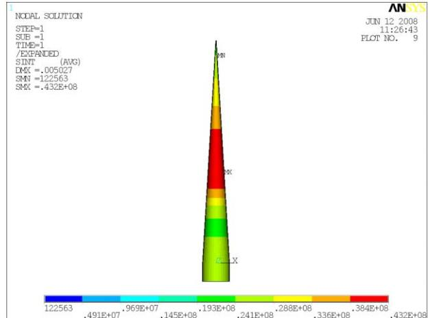
Figure 6: Total Tresca stress intensity for actual design.
