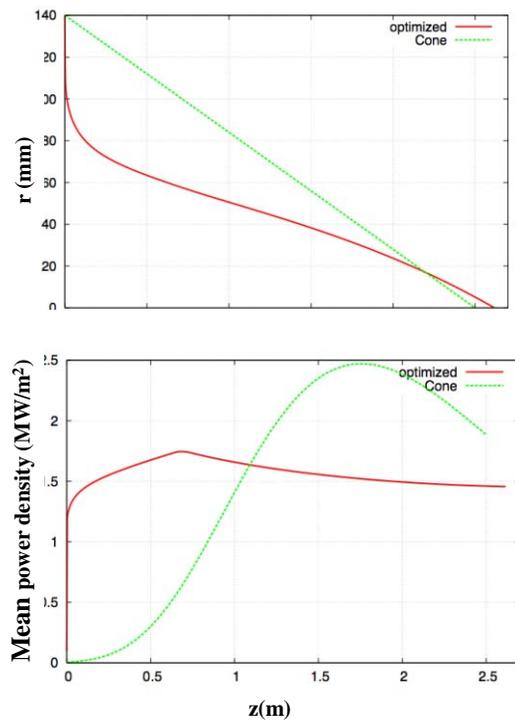
Figure 2: Mean Power density deposited at a conical beam dump (green lines) and at a beam dump with the same length and minimum peak power density (red lines).
