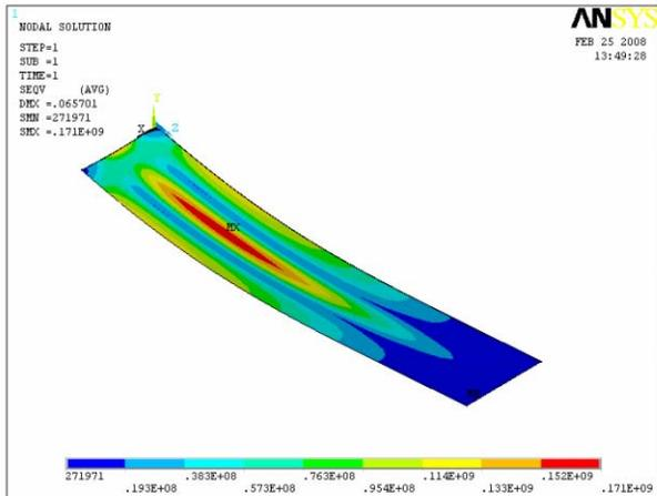
Figure 5: Von Mises stress for plate geometry.
