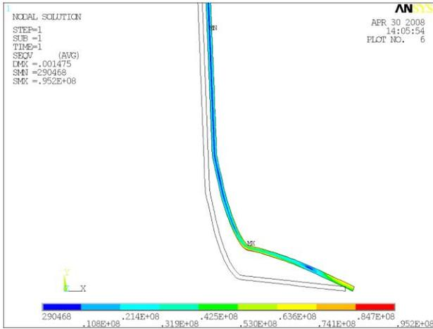
Figure 4: Von Mises stress at the base of the optimized geometry. Section view, beam direction vertical upwards
