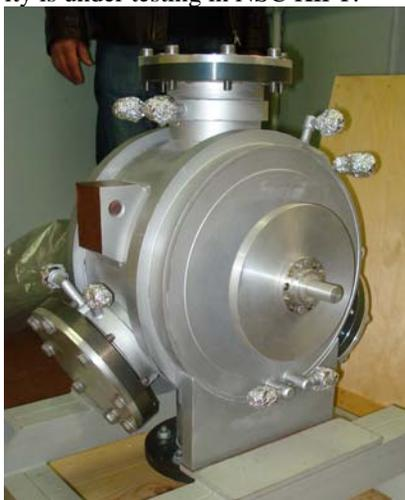
Figure 4. View of the assembled accelerator of NESTOR RF cavity.
