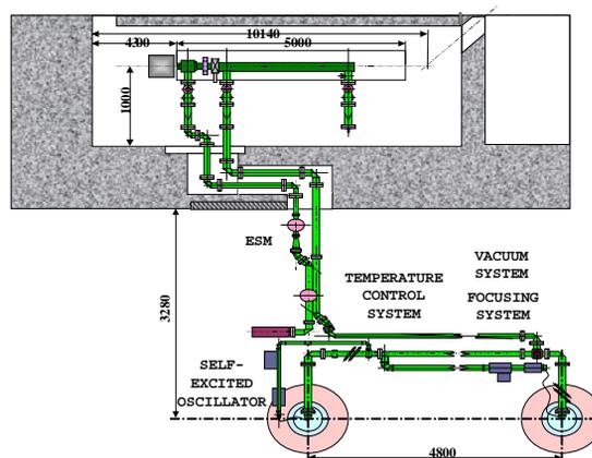
Figure 1. Layout of the NESTOR linear accelerator injector.
