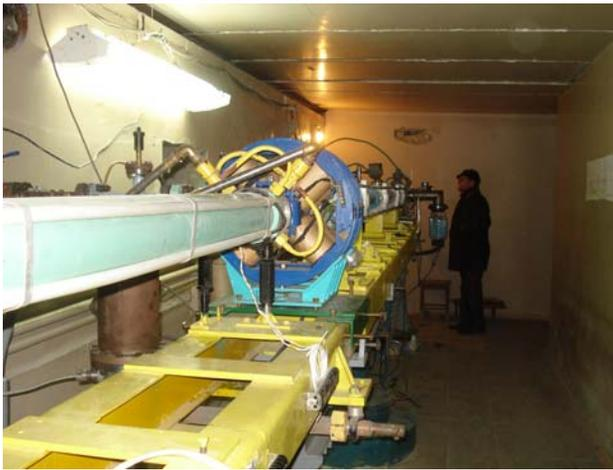
Figure 2. View of the assembled accelerator of NESTOR facility.
