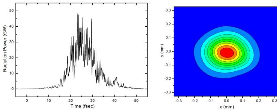
Figure 3: Simulated XFEL beam output at 1 Å. (left) Temporal intensity variation, FWHM is 20 fsec in this case. (right) cross-sectional X-ray intensity profile at 50 m downstream from the undulator (SIMPLEX simulations).
