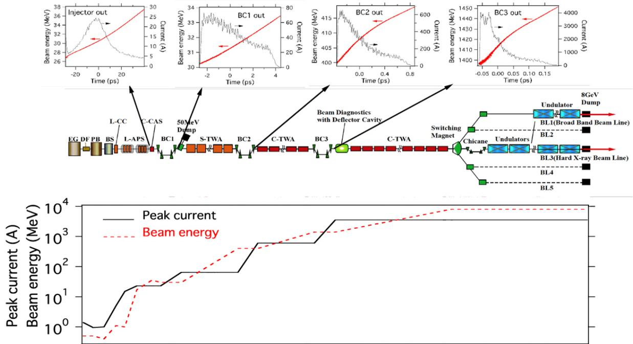
Figure 2: Machine configuration and beam current v.s. energy profile along the accelerator. Three chicane bunch compressors will be implemented, where the peak current will be increased step-by-step as proportional to the beam energy increase.
