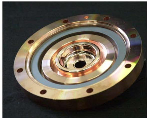
Figure 4: (left) Four C-band accelerating structures are installed in the SCSS test accelerator. Two of them are running at 36.6 MV/m in daily operation, providing beams for user experiments. (right) C-band accelerating structure is made by 92 cells made by OFC copper. The black coloured ring is SiC, which absorbs higher order modes excited by passing electron bunches, which enables low-emittance multi-bunch beam acceleration..
